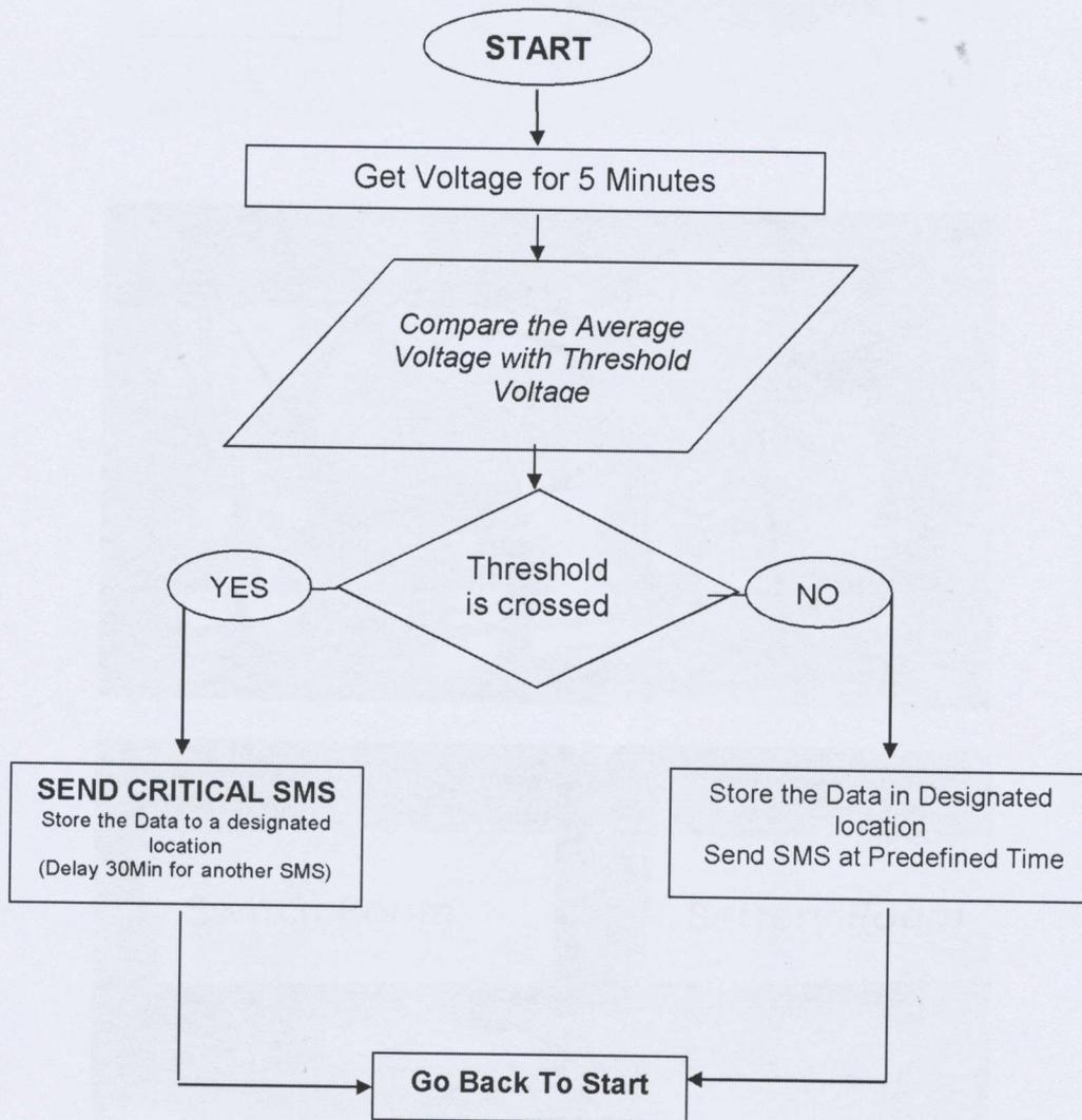
Figure: Block Diagram of the DVMAS
