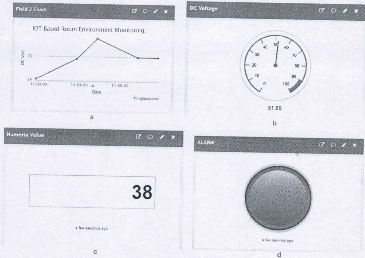
Figure: DVMAS OVER INTERNET (a) Graphical Representation of Voltage with time; (b) Continuous Voltage Meter with Critical(Marked RED); (c) Numerical Display of Voltage; (d) Critical Voltage Alert Light;
